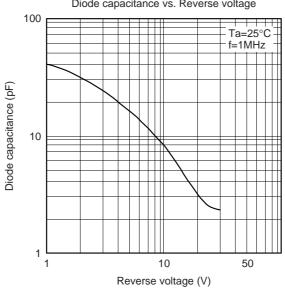
Diode capacitance vs. Reverse voltage
